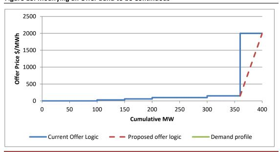
Figure 18: Modifying an Offer Band to be Continuous
