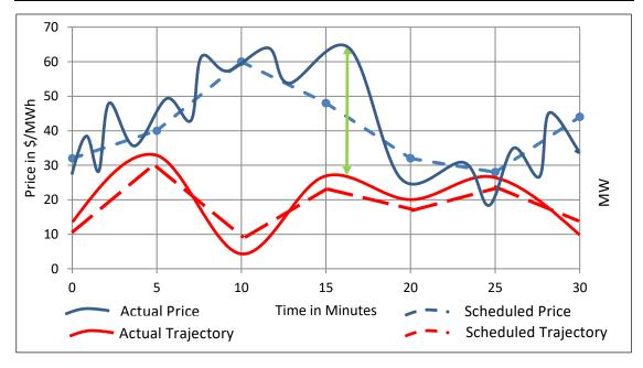
Figure 6: Load or Generation Trajectory with Real Time Pricing
