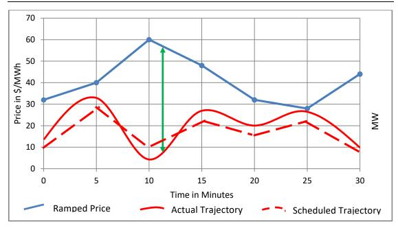
Figure 5: Load or Generation Trajectory with 5 Minute Ramped Pricing
