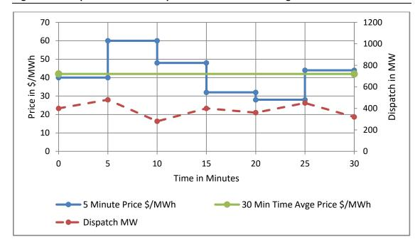
Figure 1: Example of 5 Minute Dispatch and Half-hour Pricing
